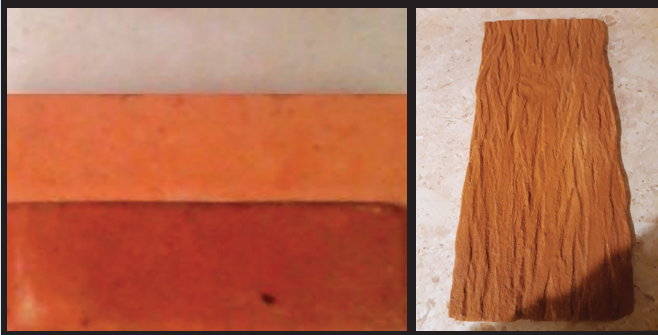
Figure 2. (left) Pigmented Neuskyns. (right) Neuskyns slab embossed with redwood bark pattern. Credit: NanoArchitech.
